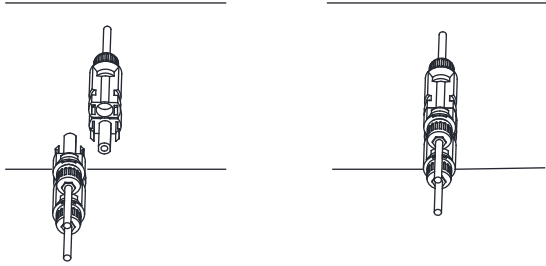
Pic 5.6 DC input connection
